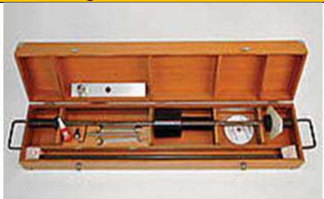
**Ductility Test Apparatus**
