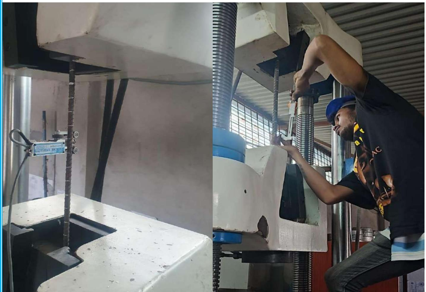
**Using Extensometer for 0.2% Proof Stress & Measuring Gauge Length at maximum Force**
