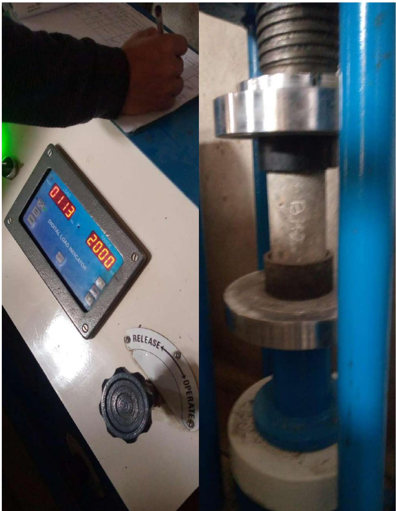
**Compressive Strength test of Concrete core with using Retainer Ring**
