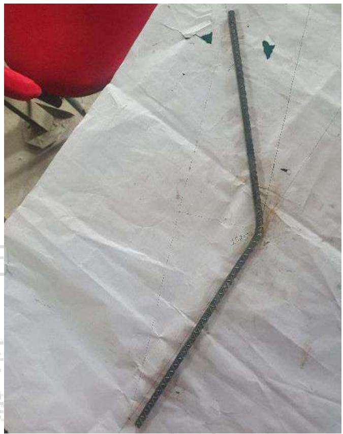
**Re-bend Test of Reinforcement bars**
