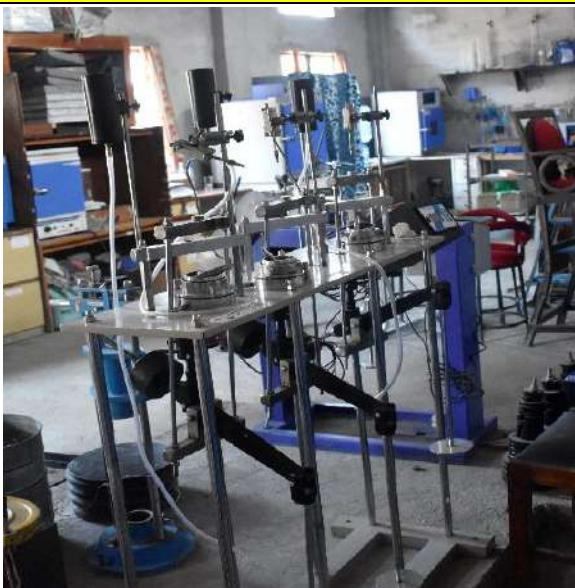
**Direct Shear Test Machine**
