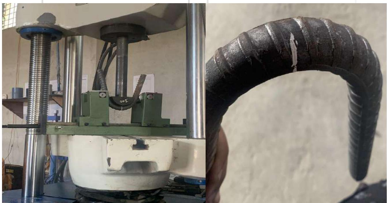
**Bend Test of Rebar**
